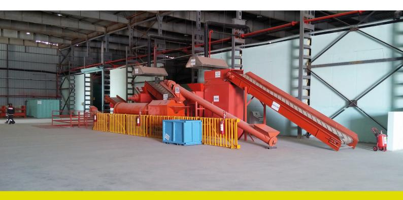
PAR 60110 can shred tires and various scrap rubber products at rates from 2-3 tons / hour (200-300 car tires).
