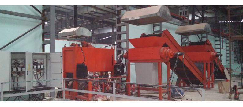
This powerful dual-shaft shredder easily handles whole passenger and light truck tires with output shreds down to 25-75 mm chips.
